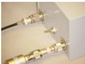
This filter allowed my fellow ham to work 160 Meters - all of 160 Meters, including the CW portion of the band right down to 1800 KHz - without the debilitating effects normally experienced by his receiver due to overload from the strong commercial AM broadcast band signals present at his QTH located in North central Texas.
